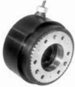
Tooth Clutches & Brakes (Electromagnetic) 2.25" - 18.7" Dia. 10 lb-ft. - 24,000 lb-ft. Many special designs available
