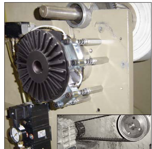
Montalvo CD100 brake replaces inefficient particle brake greatly enhancing performance of a Mark Andy press.
